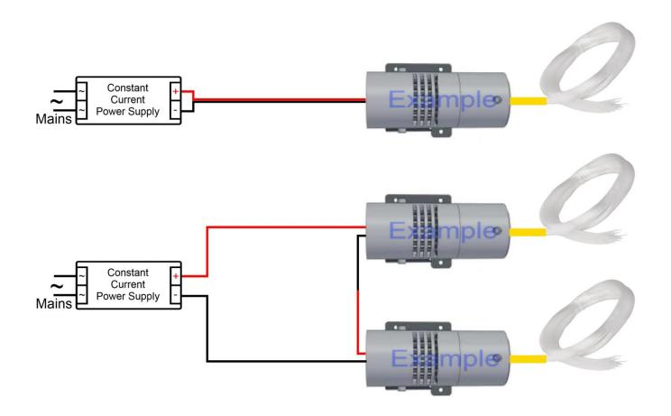
LFM can be connected only with serial wiring. LFM may be connected to driver. Above connection is examples and may be different from the actual.
